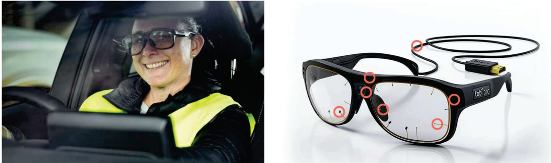
Figure 4. Real-time eye gaze data was captured with sophisticated wearable eye tracker glasses. The Tobii Pro eye tracking glasses are lightweight, unobtrusive and do not affect driving performance.
