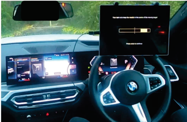
Figure 12. Stationary testing with the Tracking Task in the AARC carpark. The Tracking Task is a computer-based task that requires a laptop computer, keyboard and a windscreen mount to hold the laptop in front of the participant. The “tracking” component of the task is a continuous task that simulates driving.
