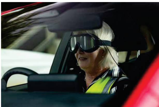
Figure 11. Visual Occlusion Test — Visual demand was assessed using vision occlusion goggles (VOGs) that limit participants' access to the IVIS. A microswitch mounted on the index finger enabled participants to momentarily "open" the goggles to view the interface during task completion. The cumulative duration of these openings represents the visual-attentional demand imposed by each IVIS.
