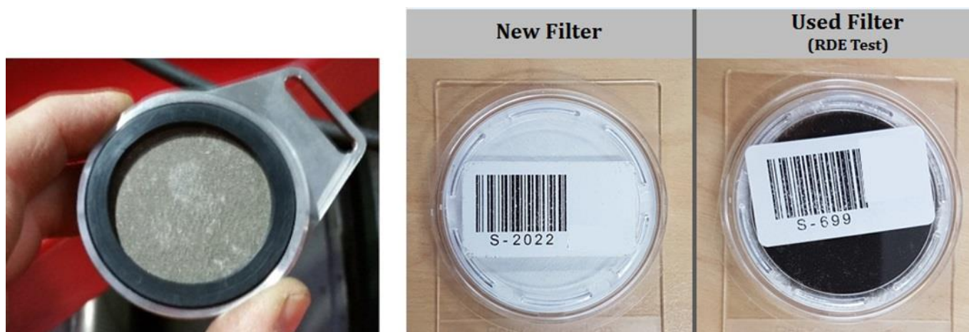
Figure 22 – (Left) Example PM Filter After Use, (Right) Example PM Filters Inside Individually Bar-Coded Petri Dishes
