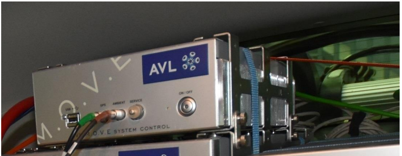
Figure 18 – PEMS Data Logger & System Control, Installed in a Test Vehicle
