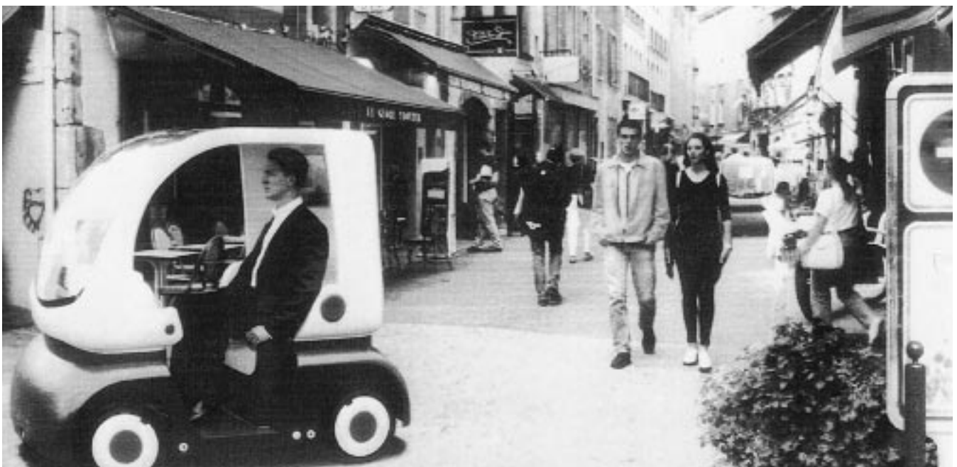
This is a prototype of a dual mode self-service car that can operate on tracks and roadways.
