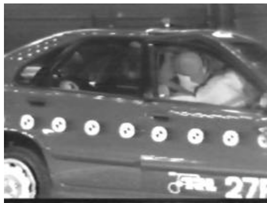
Offset crash test at 64km/h
