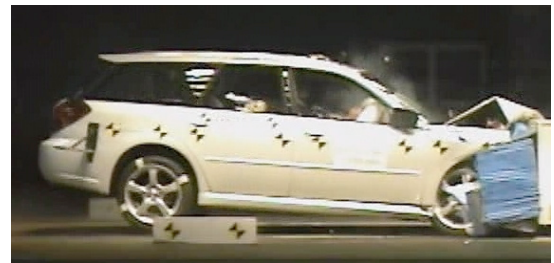
Offset crash test at 64km/h
