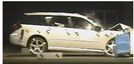
Offset crash test at 64km/h
